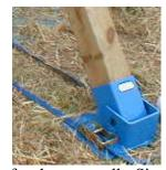
Stored in this fashion, the tool can be quickly put into service for the next call. Simply set the tool on the ground, bull the strap from the storage area, and extend the hook to the attachment point. Remove all slack by hand before engaging the ratchet.
