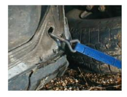
Example: Vehicle on its roof, nose down. Set your ground pads to the rear of the car. Prop to the underside of the bumper, and run the strap through the back window, around the "C" post and hook to the "D" ring.
