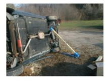
With the 4 x 4 in place as a prop, set the system by giving the back plate of the ground pad a sharp blow with your hand or foot. This will tighten the system enough to allow you the use of both hands to secure the ratchet.
